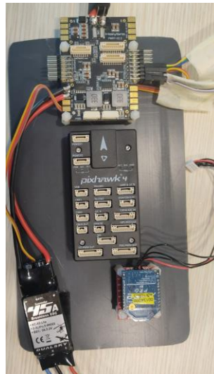
Figure 6: PDB + Pixhawk 4 + ESC + XBee mounted onto the PVC
