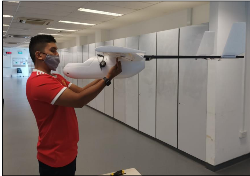
Figure 56: Side View of CG testing with 2 points on the wing
