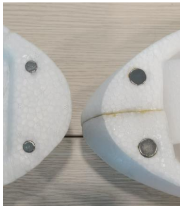
Figure 10: Magnets used to secure the nose cover
