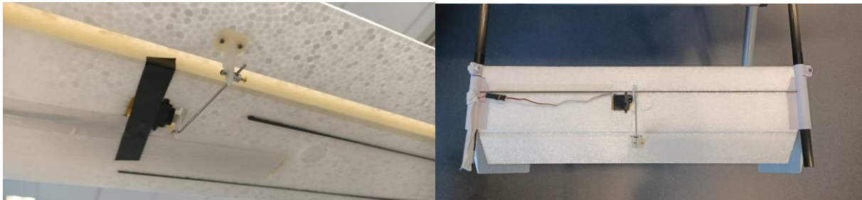
Figure 7: Servo motors mounted on the wings + elevator
