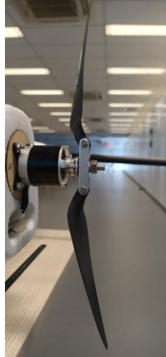
Figure 5: Motor mounted at the rear of the fuselage with propellers mounted to the motor hub
