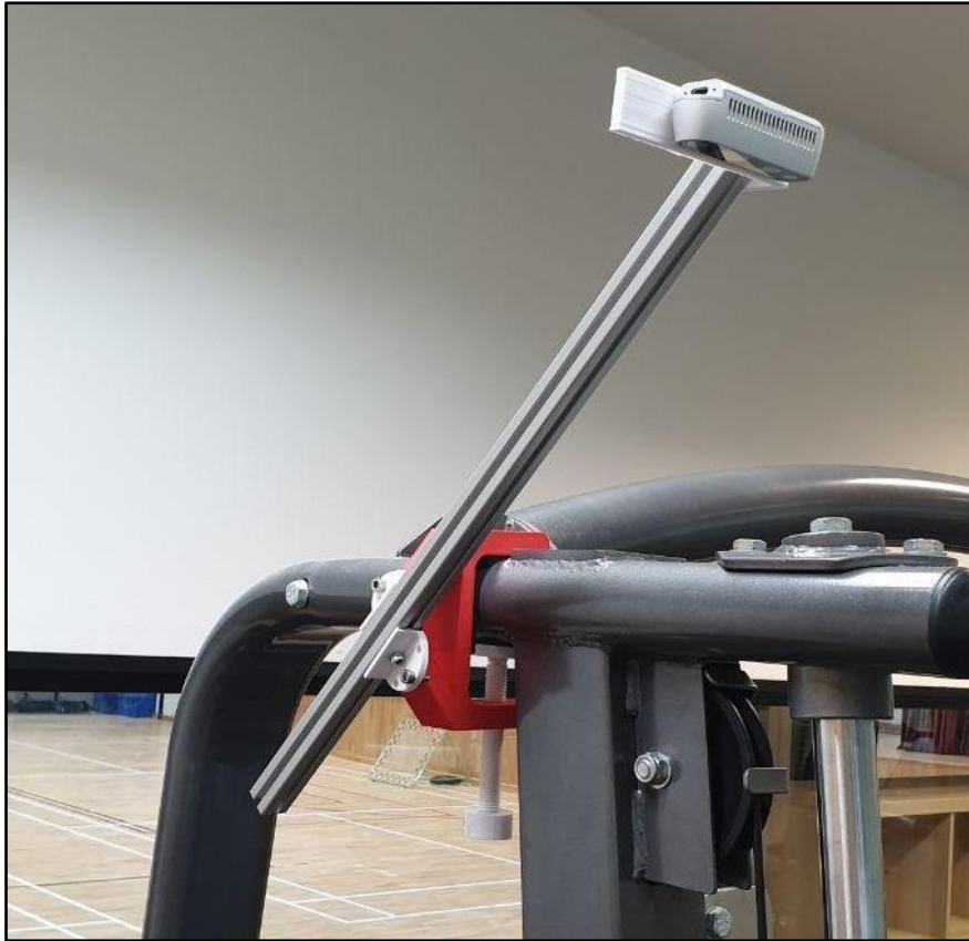
Figure 4.1.9: First Iteration of the Camera Mount System
