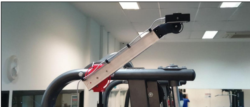
Figure 4.3.5: Final Iteration of the Camera Mount System (Side)
