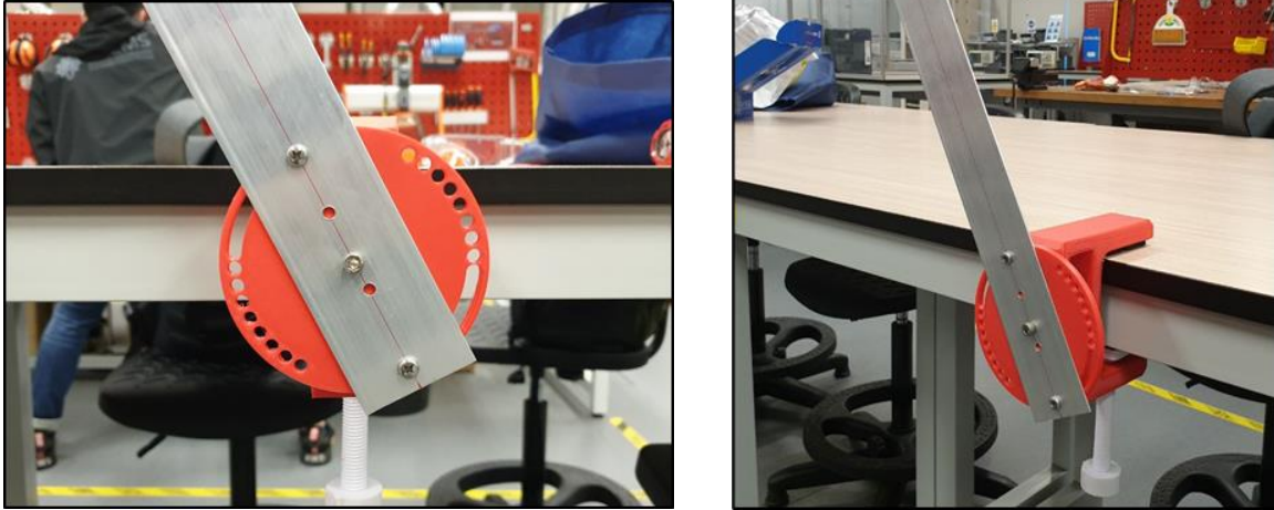
Figure 4.2.3: Aluminium Plate Cantilever Arm with Angle Locking Rotary Dial
