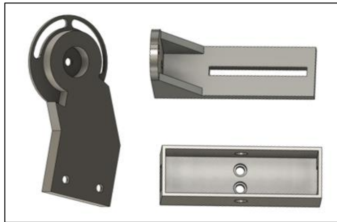
Figure 4.3.2: CAD Models of Modified L-Bracket and Camera Housing
