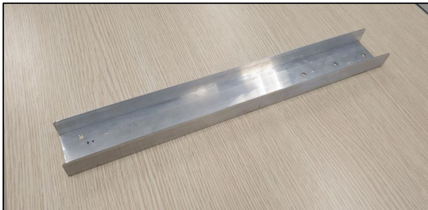
Figure 4.3.1: Fabricated C-Channel Cantilever Arm
