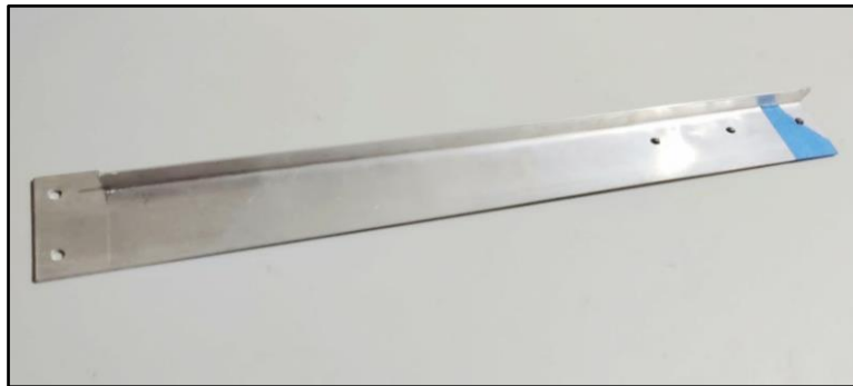
Figure 4.2.4: Fabricated L-Shaped Cantilever Arm
