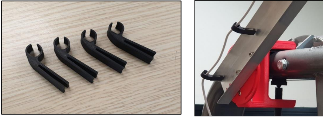
Figure 4.3.4: 3D Printed Slide-On Cable Guides (Left) Fitted onto Cantilever Arm (Right)
