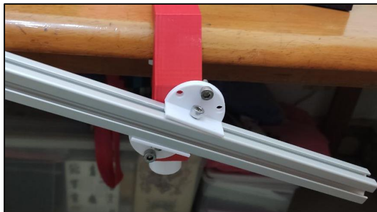
Figure 4.1.8.: Double Angle Locking Mechanism
